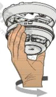
Fig. 1 - Alarm indicator (AI) centered in the detector; no alignment required
